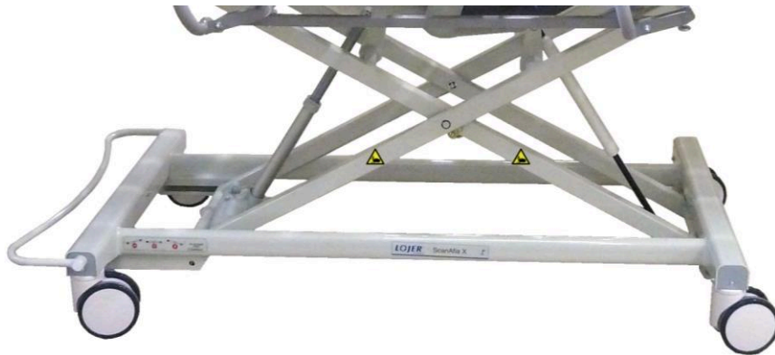
Figure 43. Danger of crushing in the scissor structure of the bed
