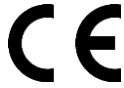
Figure 10. Product or component marked with this symbol meets the requirements of directive 93/42/ETY (medical devices) and its current amendments.
