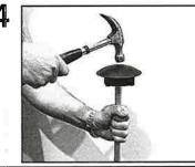
Very Important: Firmly hit the sphere with a hammer or turn upside down and hit firmly against the floor to lock into place.
