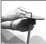
Again using the Allen Key, tighten the screw to lock the flat disc in place.
