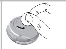
Put the battery into the battery compartment in such a way that the battery is on top of the spring underneath the clip (1) and the positive pole (+) faces upwards.
