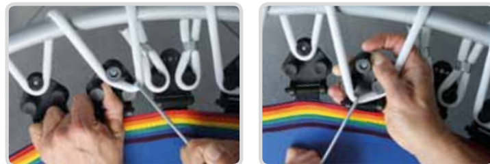
Raising the tension from position 1 to position 3
