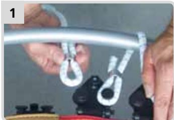
Hook the end of the cable to be used onto the free tensioning element.
