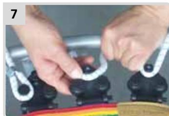
Feed the cable around the desired cone at the next tensioning element.
