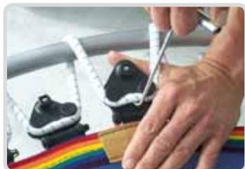
Tension is increased further by changing the routing from position 3 to position 4
