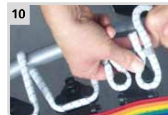
Hook the end of the cable onto the last tensioning element.
