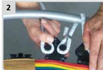
The 2 cable lengths which lead to the tensioning element should both always be fed above or below the frame.
