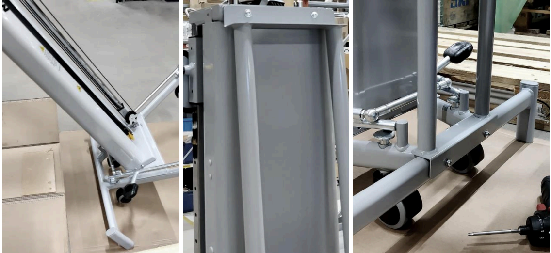
Image 13. Lifting up the device and attaching the back support
