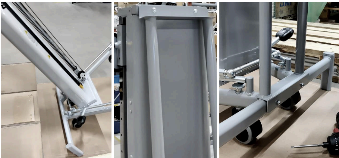
Image 13. Lifting up the device and attaching the back support
