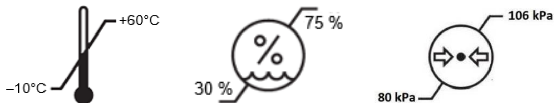
Image 4. Symbols and limit values for transport and storage temperature, humidity and atmospheric pressure.
