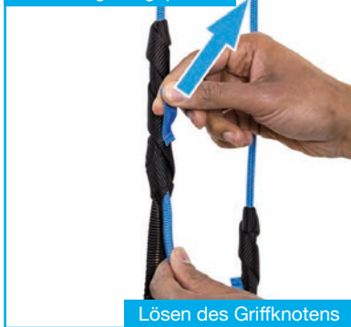
Moving the grip knot downwards
