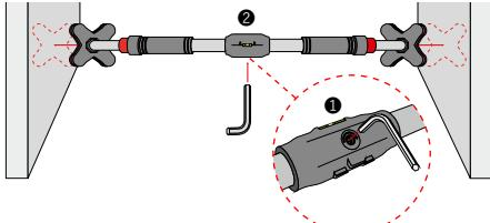
Adjust the length of the pull-up bar to the width of the door frame by turning the adjustable screw ①. Use an Allen wrench for this. The adjustable screw is located on the underside of the centre section ②. Turn it until the bar makes contact with the door frame.
