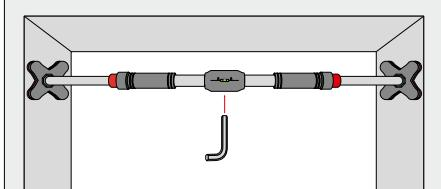
Now turn the adjustable screw until the bar is firmly seated in the door frame.
