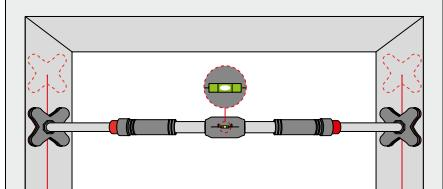
Now push the pull-up bar up to the desired position of the door frame. Make sure that the bar is placed horizontally in the door frame. The built-in water level makes it easier for you to align.
