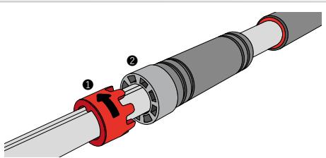
Place the pull-up bar on the floor in the desired door frame. Unfasten the two red clamps ① from the grip ends ② and pull them outwards so you can adjust the length of the pull-up bar.
