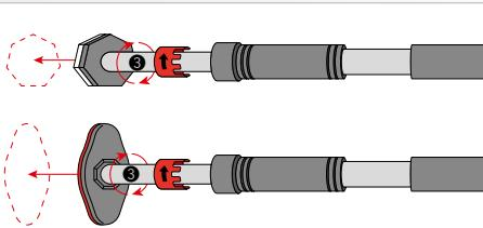
Now adjust the length of the pull-up bar to the width of the door frame by unscrewing both ends of the pull-up bar ③ until the bar is in contact with the door frame. Be sure to unscrew both ends evenly.
