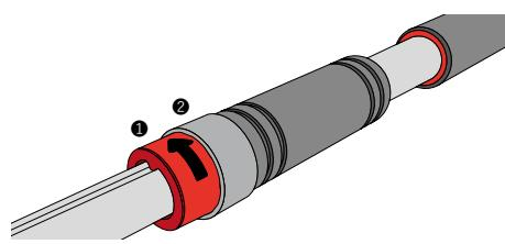
Put the red clamps ① on the grip ends ② on both sides to secure the pull-up bar. Make sure that the pins of the clamps fully engage with the receptacles on the bar. To do this, it may be necessary to twist the bar a little more.
